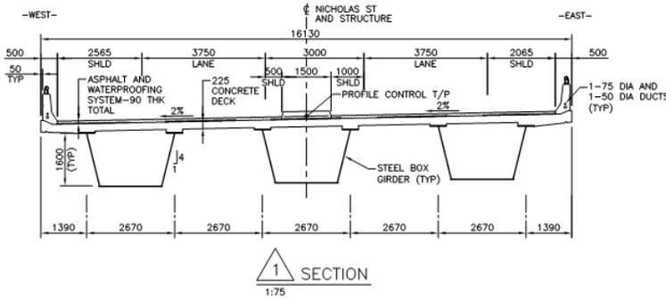
Figure 2. Superstructure cross section
