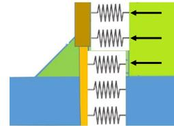
Figure 5. Imposed displacement on soil springs
