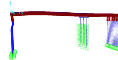
Figure 6. Deformed shape of the bridge and pile foundations under lateral spreading (exaggerated)
