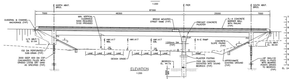
Figure 1. Bridge elevation view
